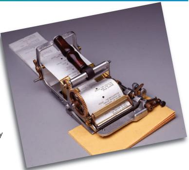
Tension of the knife return is regulated by the clutch on the left side of the machine. If the knife arm sticks and does not return after the label is cut off, push the clutch forward and clockwise to increase the return tension. Then check the knives to make sure they are adjusted correctly.
