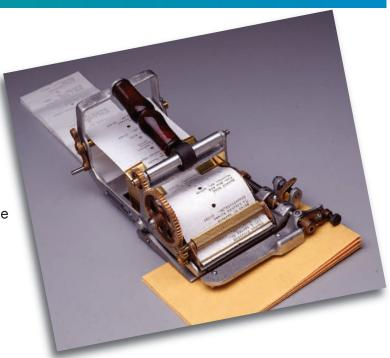
The smooth operation of your machine depends greatly on using proper adhesive, which should be fine and thin - about the consistency of very thin molasses or #20 motor oil. If too thick, it may clog the rollers; if too thin, it may ooze out from under the labels.
